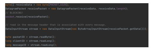
Fig. 1. Part of the Server class, this example code shows part of the code that uses a Datagram Packet to
